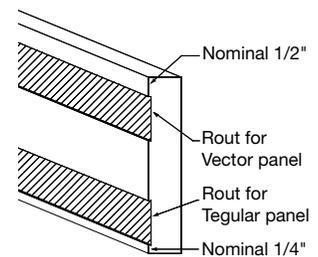
For full sized Woodworks Tegular panels using 9/16" grid, cut a miter on each end of each side of the trim so the measurement from long point to long point is 1 15/16" larger than the nominal dimension of the cloud.
