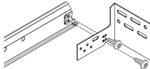
Screw the Trim Clip to the tee at these points for alignment. When the other face of the clip is against the trim, just the override of the tee will sit on the face of the molding. This is the correct spacing for full panels.
