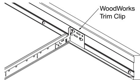
When a full sized XL cross tee meets the molding at the perimeter, line up two holes in the Trim Clip with the two "stake" holes in the end of the cross tee.
