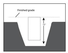
Excavate trench according to designed lighting plan, 20" deep and 10" wide suitable for the 13" fixture housing.
