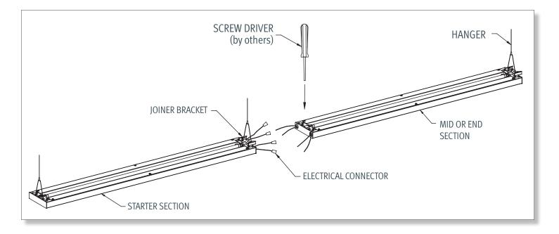
**<u>STEP 1</u>** Install JOINER BRACKET to the Joiner End of the START or MID SECTION.
