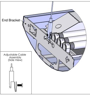
Slide adjuster clip into slot on end bracket. Secure machine screw to adjuster through the holes in the clip, tighten screw, but leave enough of a gap in the clip to slide back and forth. Slide cable though adjuster. Repeat on the opposite end for 1st fixture of row or stand-alone fixtures. For multiple fixtures, level 1st fixture, hang 2nd and level, etc. Level the complete row prior to tightening all the screws.
