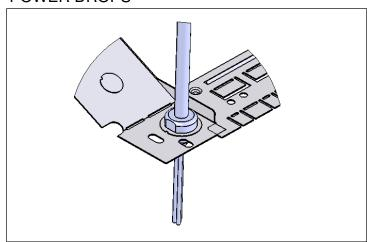
Break off appropriate KO, slide power cord through KO opening, then secure power cord with strain relief.
