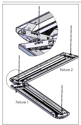
Install first fixture with two AC cables. then second fixture with one additional cable.
