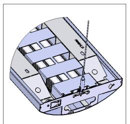
Remove film from optic before installing. To install - set in place over lamps.
