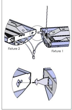
Bend out tapered aligning tabs and fit into aligner slots. (Fixture 2 is now supported by Fixture 1 at the joint.) Make electrical connections.
