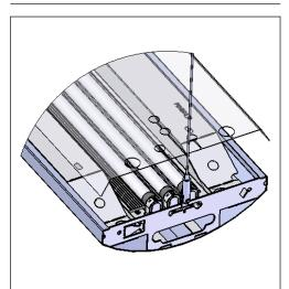
Remove film from dust cover. Squeeze dust cover into fixture. NOTE: Power cord and cables will slide through end of dust cover.
