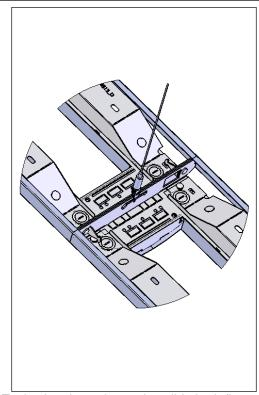
Tuck wires into wire cavity, slide both fixtures together and secure tightly using two 10-32 x 3/8" screws, starwashers and nuts. Tighten 1/4 turn past hand-tight. Starwashers must break the paint for proper grounding to occur.
