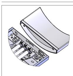
Align End Caps with end bracket of fixture. Secure using two 10-32 x 3/8" self-tapping screws.
