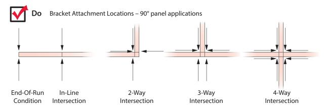
Storage-to-Panel Bracket must align with the mounting slots in the Compose full panel frame. For use in 90 degree panel intersections.
