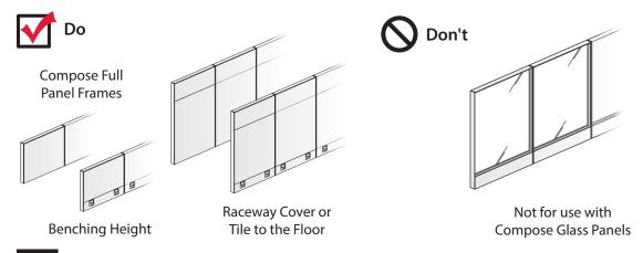
• The 297/16" high bracket (BZBG-0003) is not for use with Compose Benching height panel.
