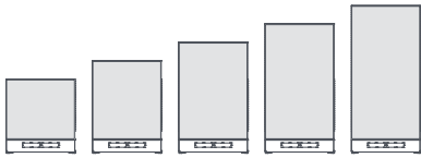
Preconfigured Monolithic Panels Monolithic panel widths: 24, 30, 36, 42, 48, 54, 60, 72 Monolithic panel heights: 32, 40, 48, 56, 64
