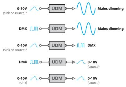
The UDM houses a mains dimmer based upon an Insulated Gate Bipolar Transistor (IGBT) to deliver mains dimming for loads up to 1000W.
