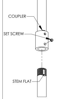
For a long overall, attach the stem segments with supplied coupler. Allign flats on stem to set screws and securely fasten.
