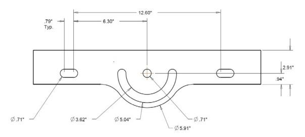
2. Use appropriate bolt size to mount either method. Secure and torque per selected bolt specifications.
