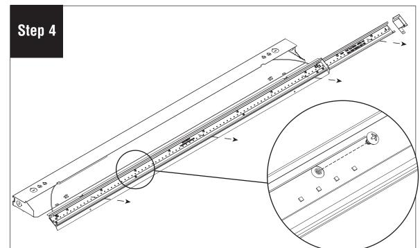
Remove all Philips #2 screws securing the light engines. Replace with new light engines. Carefully reinstall screws. Avoid any contact with LEDs during this process! Return spent light engines to Finelite or local e-waste recycler.
