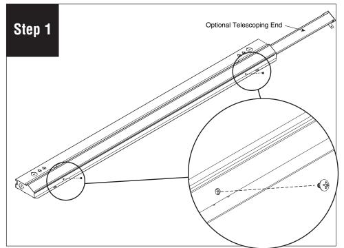
Confirm which light engines need to be replaced. Shut off power to the fixture. Remove Pull cover assembly away from body, remove endcap from telescope end and Philips #2 screws (2 per 4' fixture) on cover using #2 Philips screw driver. If fixture has telescoping end remove screws on the end that secure the endcap.
