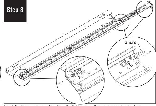
Carefully disconnect wire plugs from the light engine. Depress the locking tab to release before unplugging. Be sure to retain the end shunt (wire loop) and re-use with new light engine.
