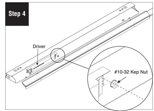
Carefully replace wires connected to Power Supply. Replace #10-32 Kep Nut with 3/8" Nut Driver to secure Power Supply to housing.
