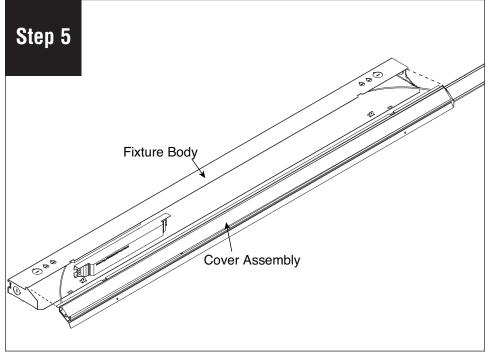
Return cover assembly and secure 2x phillips screws on cover using #2 phillips
