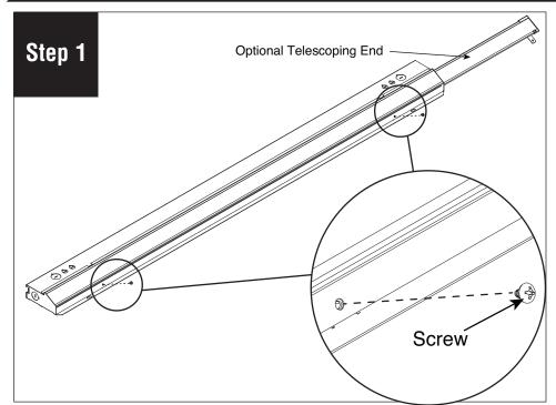
Confirm which Power Supply needs to be replaced. Shut off power to the fixture. Remove 2x Phillips screws on cover using #2 phillips screw driver.
