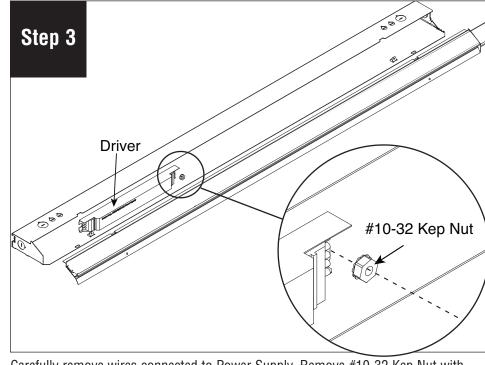
Carefully remove wires connected to Power Supply. Remove #10-32 Kep Nut with 3/8" Nut Driver, and remove Driver from Housing. Return spent Power Supply to Finelite or local E-Waste Recycler.
