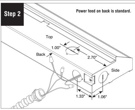
Power feeds may be located on top, back, or side of fixtures. Feed on back is standard.
