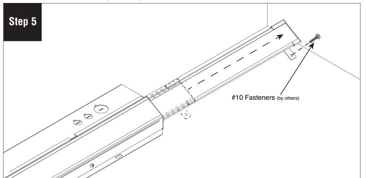
If your fixture is equipped with a 12" telescoping end option, extend this section outward to fill the cove as needed. Secure this section also using an appropriate #10 fastener by others.
