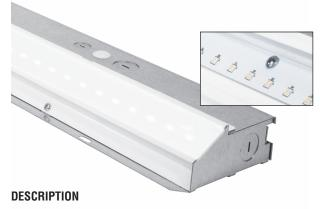
The Series 11 LED Micro Profile Cove is a high performance luminaire with an optional telescoping light engine to achieve a custom fit with continuous, uniform illumination. It is available in three color temperatures - 3000K, 3500K, and 4000K and comes in 2', 3', 4', and 8' lengths.
