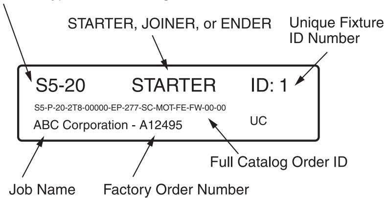
Hang fixtures in ID order. Hang prior to joining. Hang, Level, Join, repeat to the end of the run.
