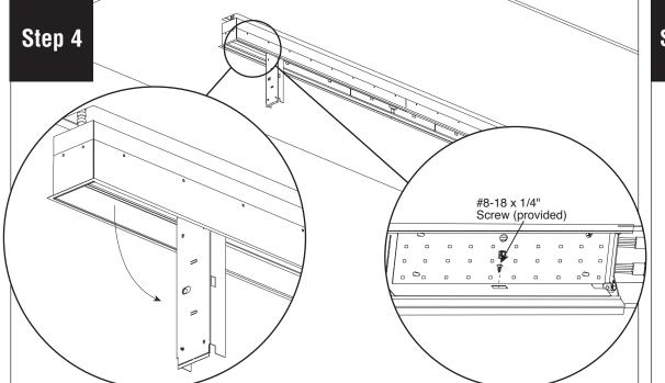
Remove #8-18 x 1/4" screw (provided) to open trap door and then insert fixture into ceiling. Align fixture within rough opening in drywall and 1/4"-20 All-Thread.
