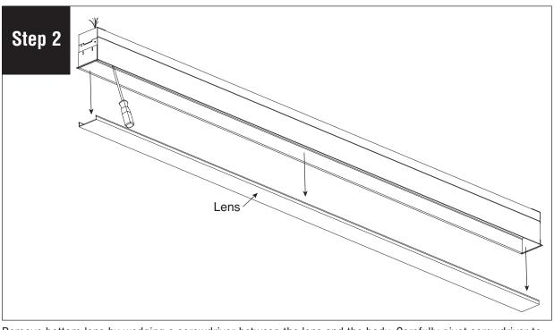
Remove bottom lens by wedging a screwdriver between the lens and the body. Carefully pivot screwdriver to unsnap the lens from the body. Set lens aside to prevent it from getting dirty or damaged during installation.
