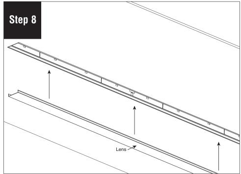
Reinstall lens and turn power on.
