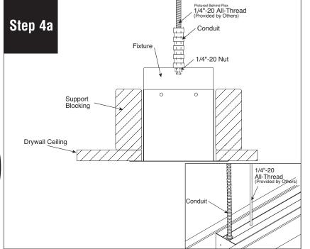
Secure fixture to structure using 1/4"-20 All-Thread.
