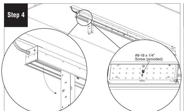
Remove #8-18 x 1/4" screw (provided) to open trap door and then insert fixture into ceiling. Align starter fixture within rough opening in drywall and 1/4"-20 All-Thread.
