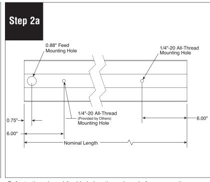
Refer to threads and feed hole locations above before connecting fixture wires.
