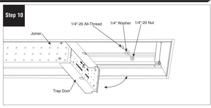
On opposite end of fixture, fold trap door down. Install 1/4" washer and 1/4"-20 nut onto 1/4"-20 All-Thread or use ALTERNATE OPTION (see step 5A). Replace trap door and fasten with #8-18 x 1/4" screws (provided).
