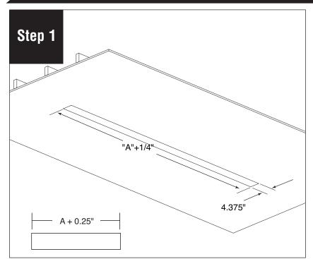
Add 0.25" to body/row length (A) +/- 1/16" to simplify installation. Fixture installed next to supporting block (optional).
