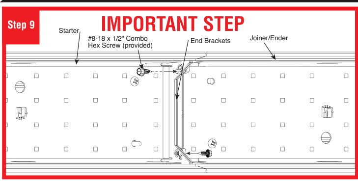
Install 2 #8-18 x 12" combo hex screws (provided) into end brackets as shown. Screws can be installed from the left or right.
