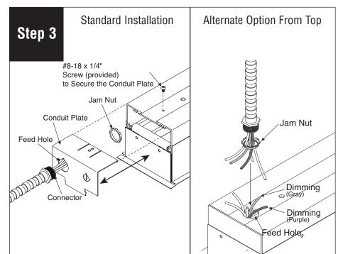
Remove jam nut from conduit then insert wires and connector through feed hole.
