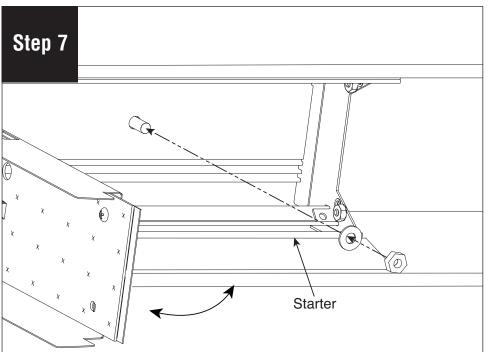
On opposite end of fixture, fold trap door down. Install 1/4"-20 nut and 1/4" washer onto 1/4"-20 All-Thread or use ALTERNATE OPTION. Replace trap door and fasten with #8-18 x 1/4" screws (provided).
