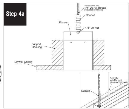
Secure fixture to structure using 1/4"-20 All-Thread.
