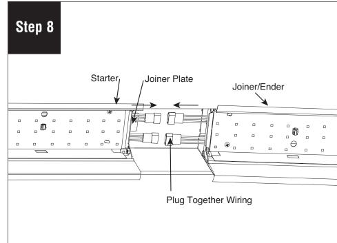
Connect plug together wiring. Slide joiner fixture against starter fixture. Be careful not to damage any wiring.
