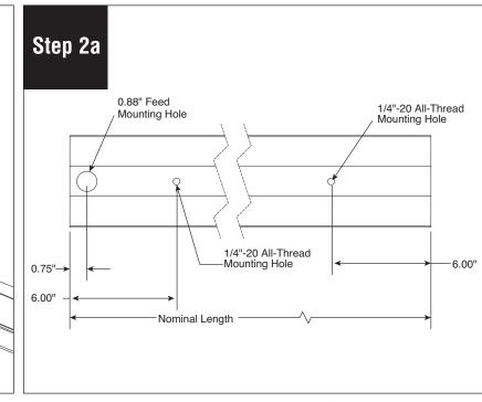
Turn off the power to the fixture's circuit. Provide rough opening according to the measurements indicated. Fixture needs to be installed next to support blocking.
