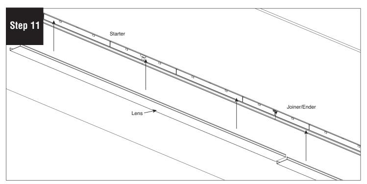
Reinstall lens and turn power on.
