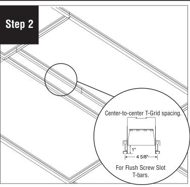
Configure T-Grid to fixture size and leave an opening for luminaire. As noted above.
