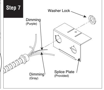
Remove splice plate from end of the fixture and insert conduit through splice plate and secure.
