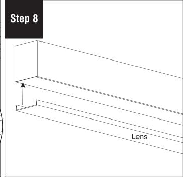
Reinstall lens and turn power on.
