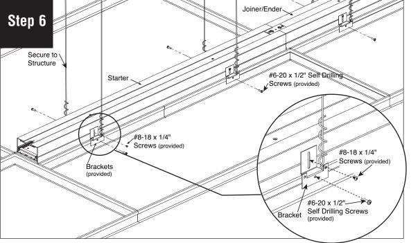
Secure all fixtures to T-Grid by driving #6-20 x 1/2" self drilling screws (provided) through brackets into T-Grid. Connect all fixtures to building structure, as per code. Use #8-18 x 1/4" screws (provided) to install brackets on fixtures
