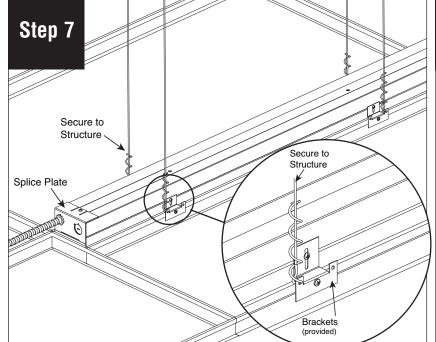
Secure luminaire to building structure, as per code.
