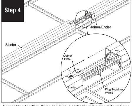
Connect Plug Together Wiring and align joiner/ender with joiner plate and carefully slide starter and joiner/ender together.
