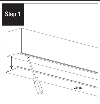
Remove lens and set aside to prevent it from getting dirty or damaged.
