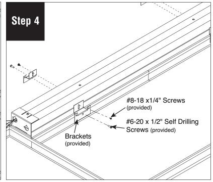
Secure luminaire on T-Grid using provided brackets and screws. Use  $\#8-18 \times 1/4$ " screws (provided) to attach bracket to luminaire and  $\#6-20 \times 1/2$ " self drilling screws (provided) to attach to T-Grid.
