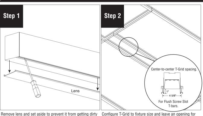
Configure T-Grid to fixture size and leave an opening for luminaire. As noted above.
