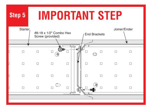
Install 2 #8-18 x 1/2" Combo Hex Screws (provided) into end bracket as shown. Screws can be installed from the left or right
