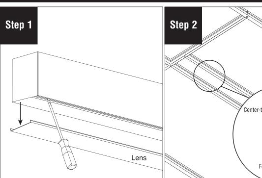
Remove lens and set aside to prevent it from getting dirty or damaged.
