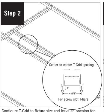
Configure T-Grid to fixture size and leave an opening for luminaire. As noted above.
