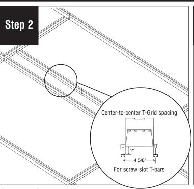
Configure T-Grid to fixture size and leave an opening for luminaire. As noted above.
