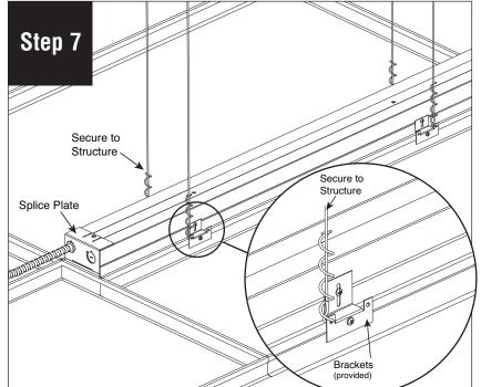
Secure luminaire to building structure, as per code.
