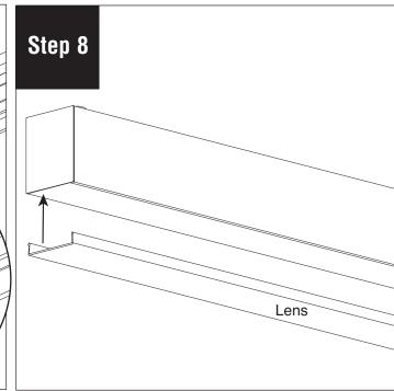
Reinstall lens and turn power on.
