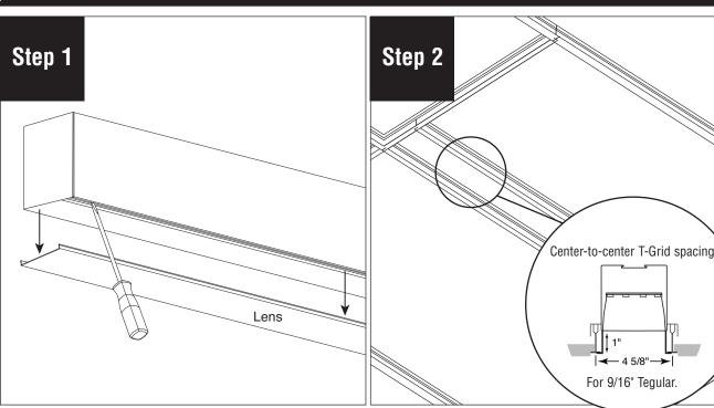
Remove lens and set aside to prevent it from getting dirty Configure T-Grid to fixture size and leave an opening for luminaire. As noted above.
