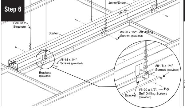
Secure all fixtures to T-Grid by driving #6-20 x 1/2" self drilling screws (provided) through brackets into T-Grid. Connect all fixtures to building structure, as per code. Use #8-18 x 1/4" screws (provided) to install brackets on fixtures
