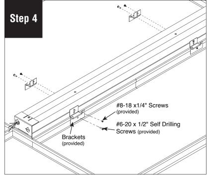
Secure luminaire on T-Grid using provided brackets and screws. Use  $\#8-18 \times 1/4$ " screws (provided) to attach bracket to luminaire and  $\#6-20 \times 1/4$ " self drilling screws (provided) to attach to T-Grid.
