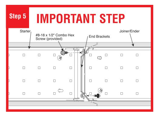
Install 2 #8-18 x 1/2" Combo Hex Screws (provided) into end bracket as shown. Screws can be installed from the left or right.
