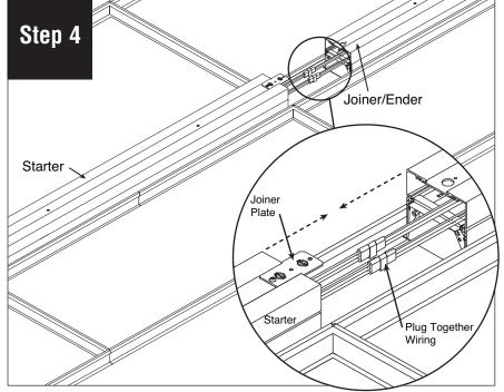
Connect Plug Together Wiring and align joiner/ender with joiner plate and carefully slide starter and joiner/ender together.
