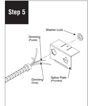
Remove splice plate from end of fixture and insert conduit through splice plate. Secure conduit with lock nut.
