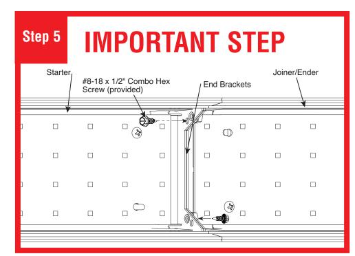
Install 2  $\#8-18 \times 1/2$ " Combo Hex Screws (provided) into end bracket as shown. Screws can be installed from the left or right.
