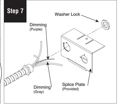
Remove splice plate from end of the fixture and insert conduit through splice plate and secure.
