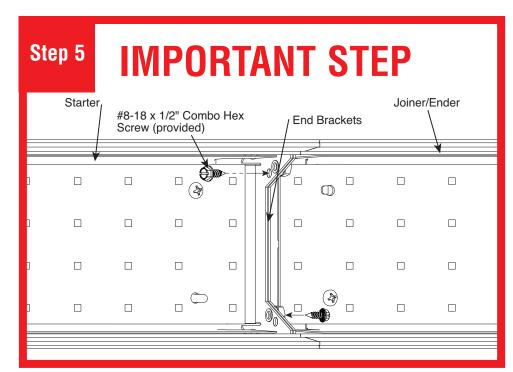
Install 2  $\#8-18 \times 1/2$ " Combo Hex Screws (provided) into end bracket as shown. Screws can be installed from the left or right.
