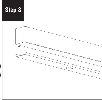
Reinstall lens and turn power on.
