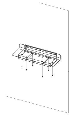
**5** Install bottom hooks by threading clockwise.
