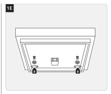
8 Mount the fixture base to the ceiling by reinstalling it on to the mounting plate and securing it tightly with the knurled nuts.
