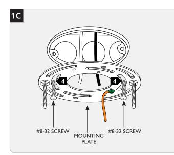
Secure the mounting plate to the electrical box with the two #8-32 screws.
