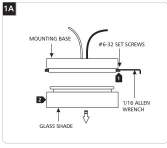
While supporting the glass shade, loosen (Do Not Remove) the four #6-32 set screws on fixture base with the 1/16 Allen wrench.
