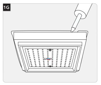
**T3** For wet location installation, caulk around the fixture base with waterproof construction sealant.
