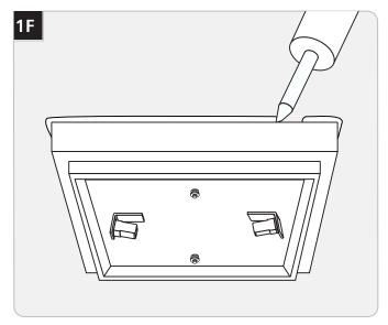
**For wet location installation**, caulk around the fixture base with waterproof construction sealant.
