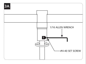
To lock the fixture head in a permanent horizontal position, tighten the #4-40 set screw on the PowerJack housing with the provided 0.05 Allen wrench.
