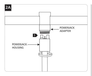
Line up the PowerJack housing with the PowerJack adapter connector and screw them together. Make sure not to cross thread.
