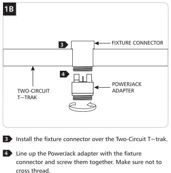
**NOTE:** In case of cross threading, unscrew the fixture connector from the PowerJack adapter and repeat steps 3 and .4
