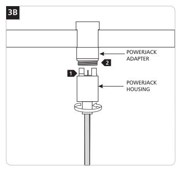
Line up and mate the socket contacts with the fixture connector contacts.
