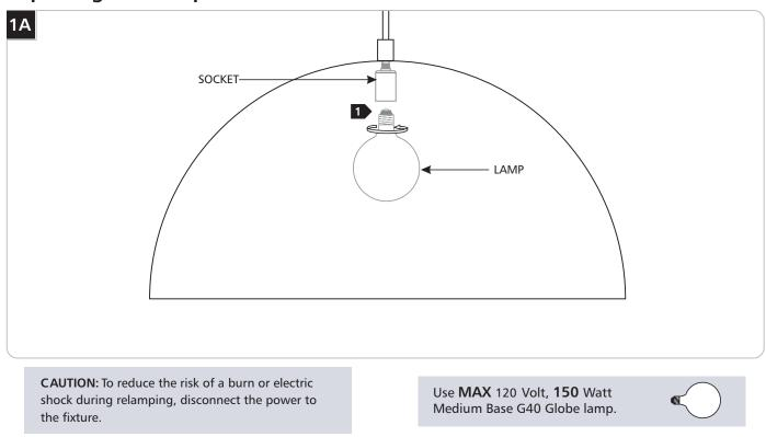
**1** Screw the lamp into the socket.
