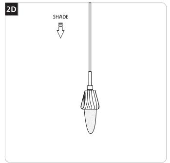
4 Lower the shade onto the socket assembly.
