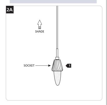
1 Lift the shade up to expose the socket.
