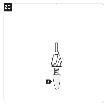
3 Screw the new lamp into the socket.
