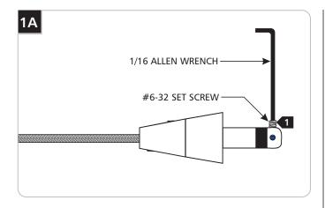
1 Back out (do not remove) the #6-32 set screw on tip of the connector with the provided 1/16 Allen wrench.
