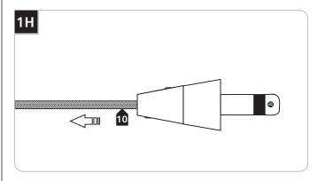
10 Pull the coaxial cable toward the fixture to smooth the wrinkles.
