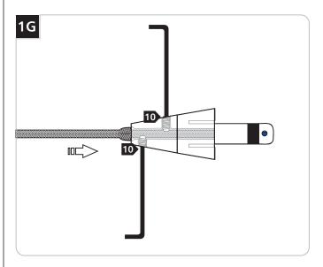
**10** Tighten the two #6-32 oval head set screws on the conical connector firmly.
