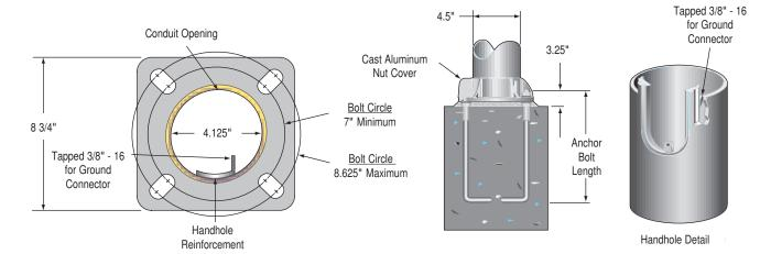
NOTE: Factory supplied template <u>MUST</u> be used when setting anchor bolts. Gardco Lighting will not honor any claim for incorrect anchorage placement from failure to use factory supplied templates.
