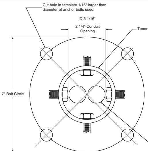
**NOTE: Factory supplied template must be used when setting anchor bolts. Gardco Lighting will not honor any claim for incorrect anchorage placement from failure to use factory supplied templates.**
