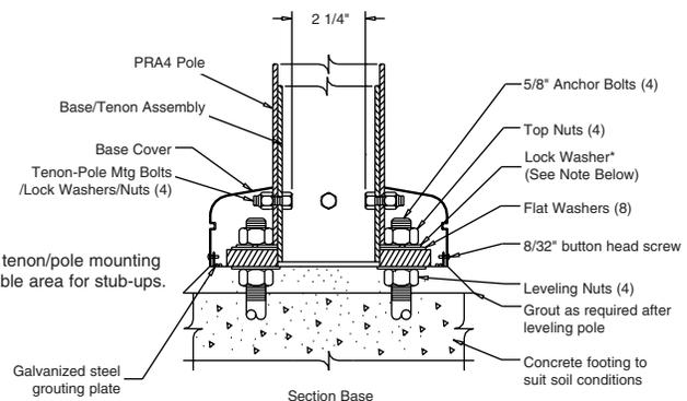
\*Anchor Bolt Lock Washers are not normally required and are not included in standard anchor bolt sets. They are available upon request at additional cost.
