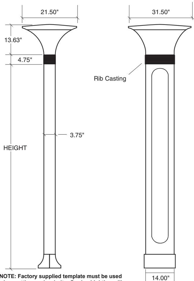
**NOTE:** Factory supplied template must be used when setting anchor bolts. Gardco Lighting will not honor any claim for incorrect anchorage placement from failure to use factory supplied templates.
