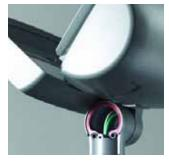
Wire splices are easily made in the spacious splice compartment, which is suitable for through-circuit wiring. No auxiliary junction box is required. Gaskets secure the wiring compartment against moisture.
