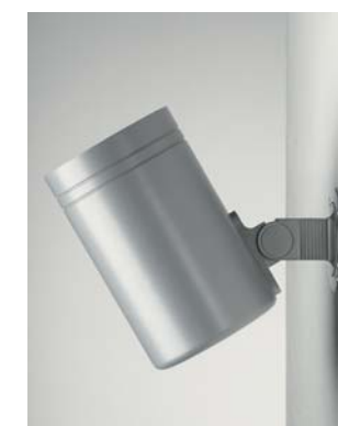
Universal knuckle for wall, ground or ceiling mount. Permits 358° rotation and 90° tilt. A cast junction box is available for pre-shipment and can be used in poured concrete or for surface mounting.
