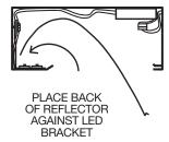
2. This will allow you to secure the LED Bracket by securing the nut(s) & washer(s) to stud(s) in housing.
