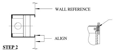
CONTINUOUS NEOPRENE GASKET MATES WITH FLANGES OF STEPLIGHT HOUSING WHEN INSTALLED PROPERLY. CAULK PERIMETER OF TRIM TO WALL TO PROVIDE PROPER SEAL TO WALL.
