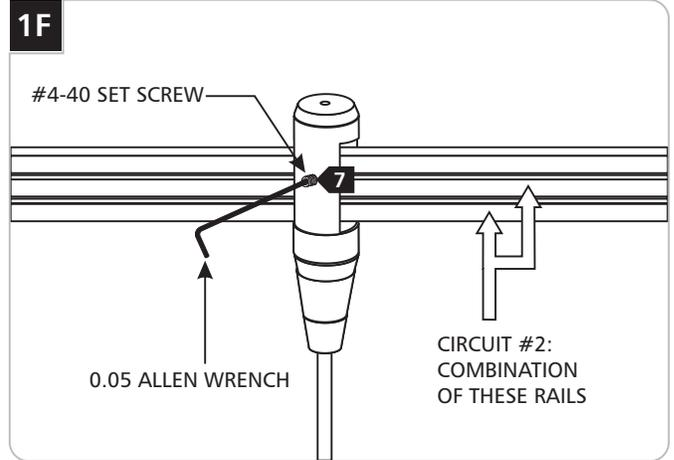
**7** When using circuit #2, remove the #4-40 set screw from top of the housing and screw it into the side with the 0.05 Allen wrench very tight.
