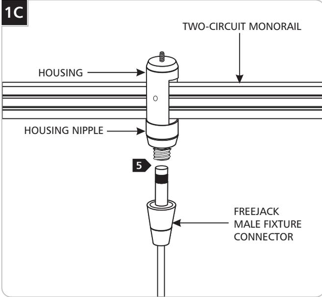
**5** Screw the FreeJack male fixture connector onto the housing nipple.
