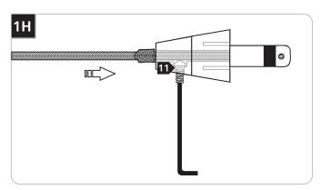
11 Firmly tighten the set screw on the conical connector.
