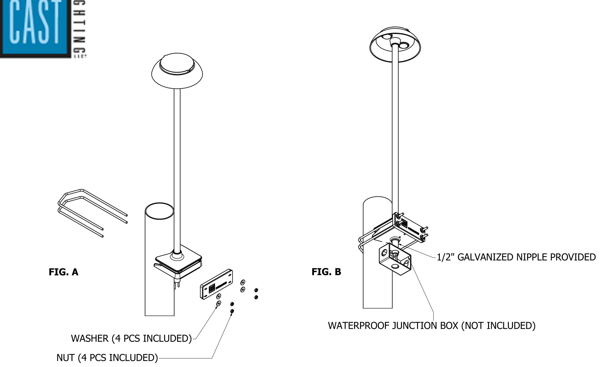
ATTACH FIXTURE TO FENCE POST USING THE HADWARE (PROVIDED) & A 7/16 WRENCH (NOT INLCUED)
