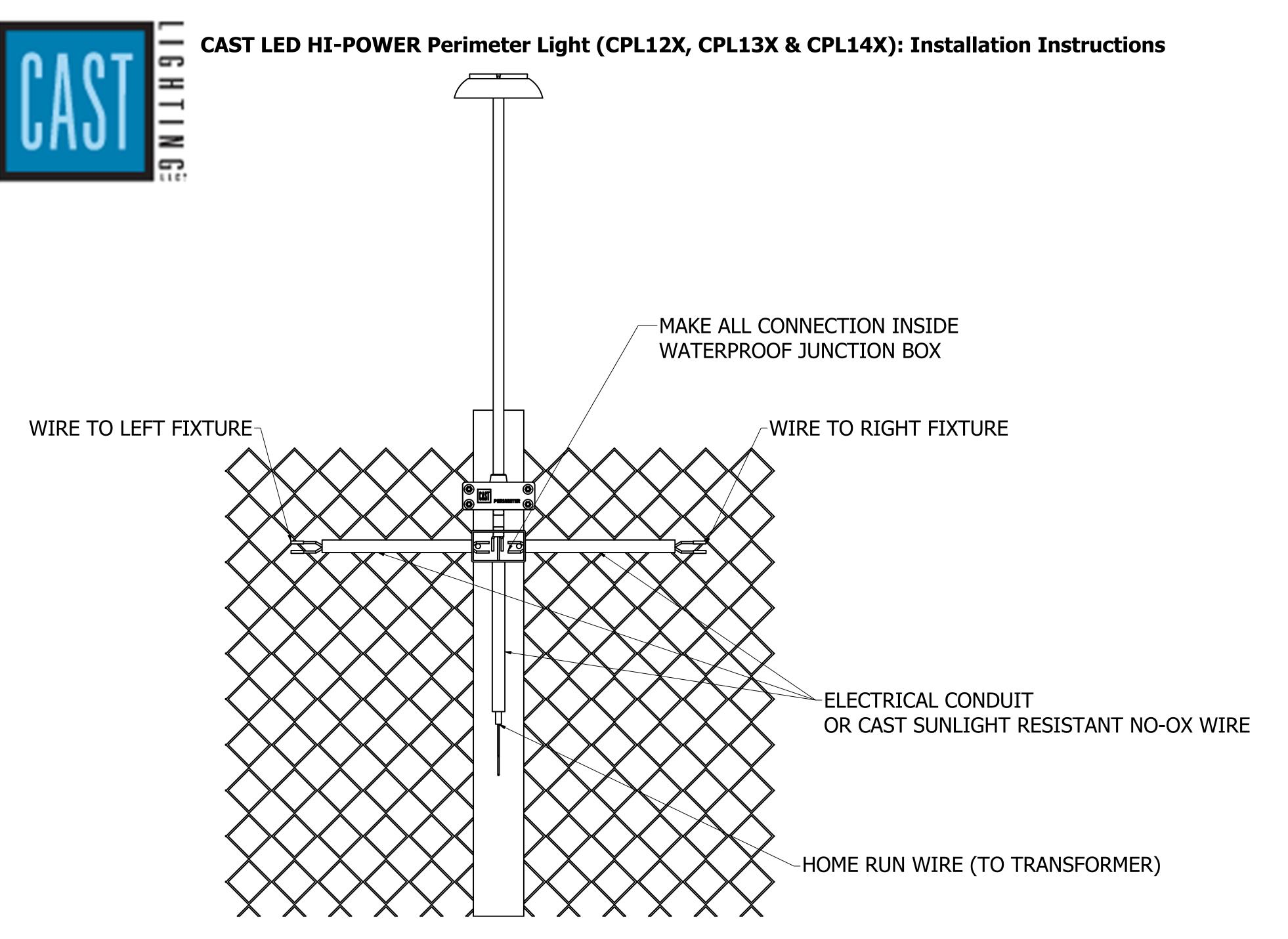
ATTACH WIRE "HOME RUN WIRE" TO CENTER FIXTURE JUNCTION BOX COMING FROM TRANSFORMER & CONNECT OTHER FIXTURES TO THE LEFT OR RIGHT AS NECESSARY.
