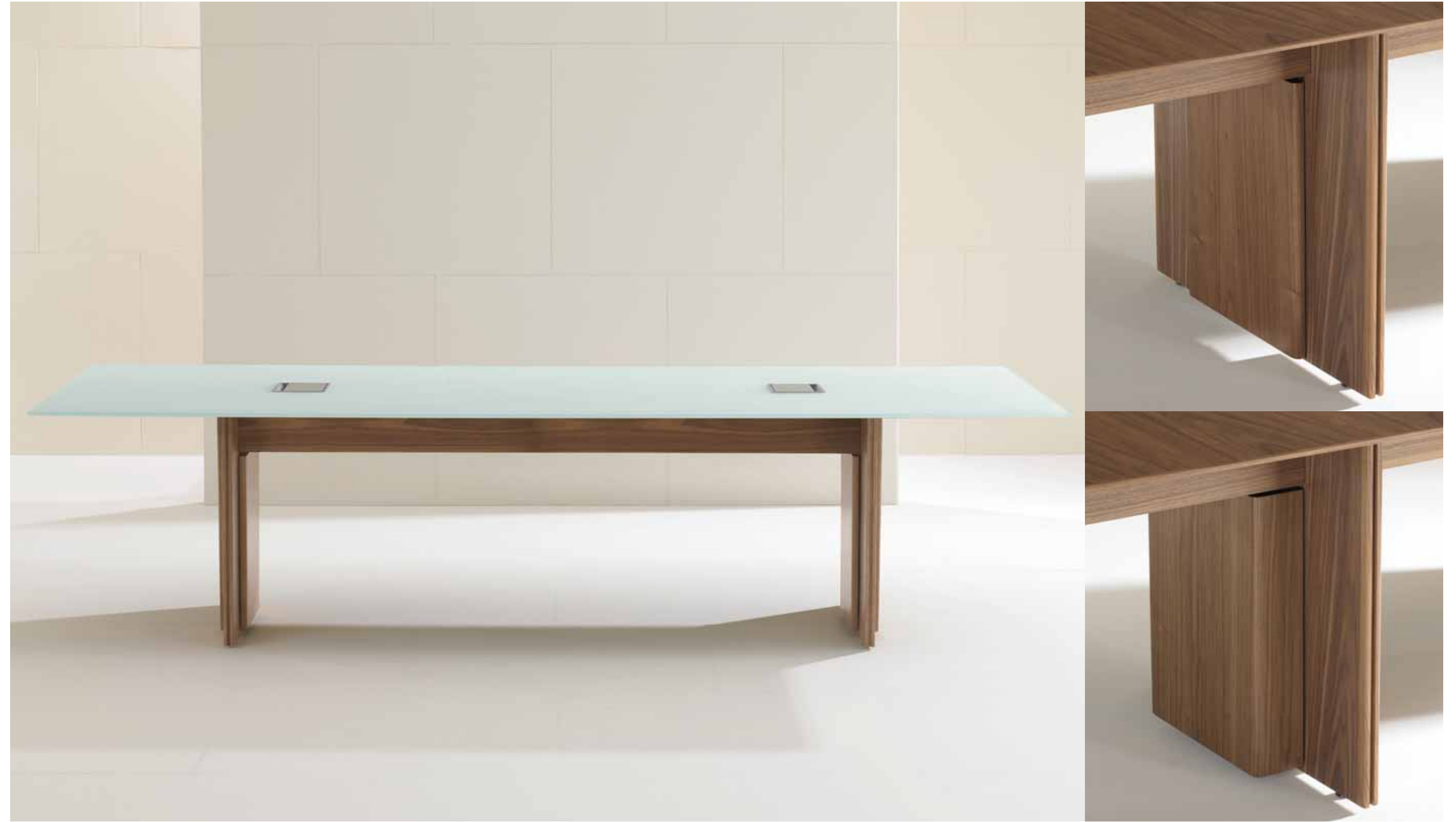
04 Opaque white, back-painted glass tops with surface sealer are 1/8" thick tempered starfire glass with polished edges. Glass tops are supported by a 1/8" thick dark brown painted sub-top that is recessed 3" from the glass edge. This glass top table, equipped with power/data access and power channel, is supported by walnut veneer panel bases.
