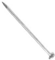
T149 Scribe Pins: Replacement pins for the Long Scriber and Short Scriber (0.063" diameter x 1.590" with brass head). Available in packs of 100 or packs of 25 (T149.25).
