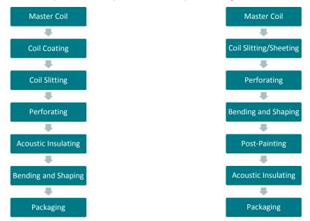
Figure 1: Typical aluminum specialty product manufacturing process, coil-coating (left) & post-paint (right)
