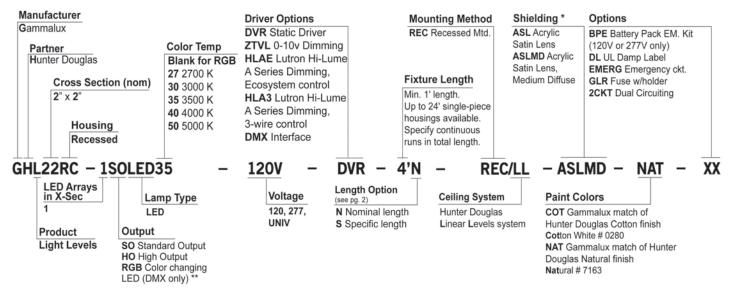
\* To better hide lamp image, medium diffuse lens is recommended. \*\* RGB lamping option must be controlled by DMX driver option.
