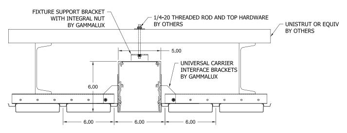
Mounting bracket is field adjustable to accommodate Box 6 or Deep Box 6 conditions.
