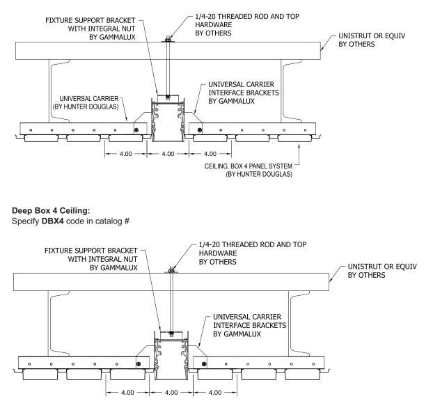
Mounting bracket is field adjustable to accommodate Box 4 or Deep Box 4 conditions.
