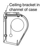
To mount against ceiling, hold screen case against ceiling and mark mounting hole locations. Each bracket has two holes towards the front edge and two holes towards the back edge. Installer must use at least two fasteners per bracket with one fastener in one of the two holes closest to back edge of bracket, and one fastener in one of the two hole closest to front edge of bracket. Installer must insure that fasteners are of adequate strength and suitable for the mounting surface chosen.
