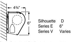
Series E Viewing Surface Shown; Series V with Tab Tensioning also available. At left, Series V slat bar is depicted inside case. Series E has a typical round bottom dowel. For all Silhouettes, the dowel is concealed inside the case.
