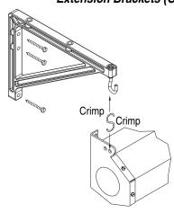
Wall mount the brackets (not included with screen) using hardware recommended for "Wall Mounting" (at right). Then, suspend the screen from the front mounting hole in the endcap with "S" hooks (as in "Ceiling Suspended"). For added safety, crimp both ends of the "S" hooks so the screen cannot come off.
