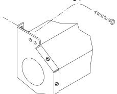
Use the holes at the back of the mounting bracket for flush wall mounting. *Recommended hardware:* For mounting into wood or wall stud, use #10 x 1<sup>1</sup>/<sub>4</sub>" wood screws; for mounting into drywall (minimum <sup>1</sup>/<sub>2</sub>" thick), use <sup>3</sup>/<sub>16</sub>" toggle bolts or <sup>3</sup>/<sub>16</sub>" molly bolts.
