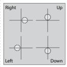
ēno interactive white-boards feature a pattern invisible to the naked eye. The pattern consists of numerous intelligent small black dots that can be read by the ēno stylus. The pattern indicates the exact positions of the ēno stylus.
