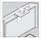
**Top-mount camera ledge** supports most industry standard HDVC cameras.
