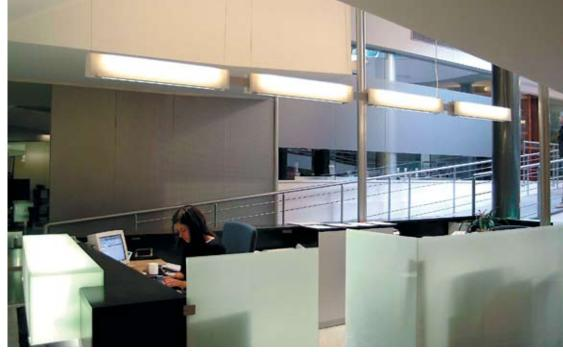
Series of luminaires with a beam form, which result from the combination of aluminum and glass. SOLIVE Suspension consists of a support in extruded aluminum and two opaline glasses attached to the sides. Polycarbonate diffusers both for indirect emission and the direct emission in the standard version. For Solive "Dark" the direct emission is controlled by a Darklight reflector. Solive hangs from the ceiling by the relevant steel wires and polycarbonate roses standard supplied.
