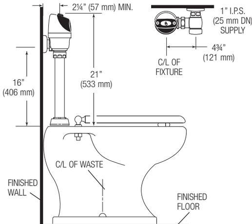
When installing the G2 Optima Plus in a handicap stall:
